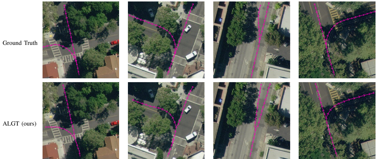
Fig. 4: Qualitative results obtained by our ALGT model in comparison to the ground truth. The top row represents the ground truth, while the bottom row presents our model’s predictions. Our proposed architecture predicts highly accurate lane graphs that do not suffer from sampled node positions as LaneGNN and shows high split detection accuracy. In general, the obtained graphs show a smooth characteristic.
