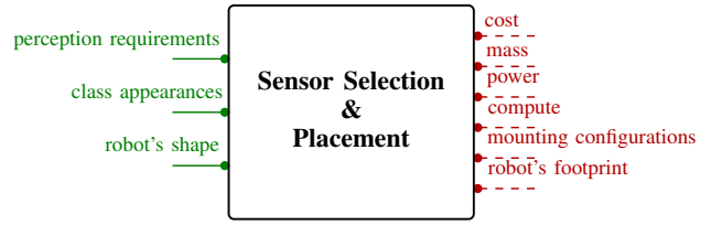
Fig. 18. The Sensor Selection and Placement MDPI which is the composition of the Coverage, Mounted Perception Pipelines and Perception Pipelines MDPIs.
