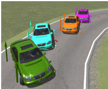
Figure 10: Animation in CarSim at time 11.5s. The green car represents HDDC, the blue car represents DDTC, the yellow car represents TMPC (ours), and the purple car represents MARTY.
