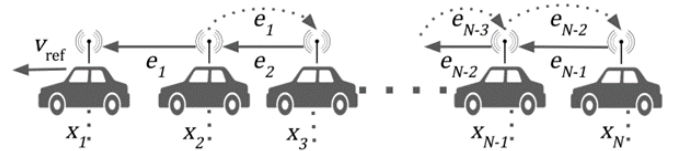
Fig. 2. Visualization of additional communication of relative position of neighbour's neighbour required to implement serial consensus.
