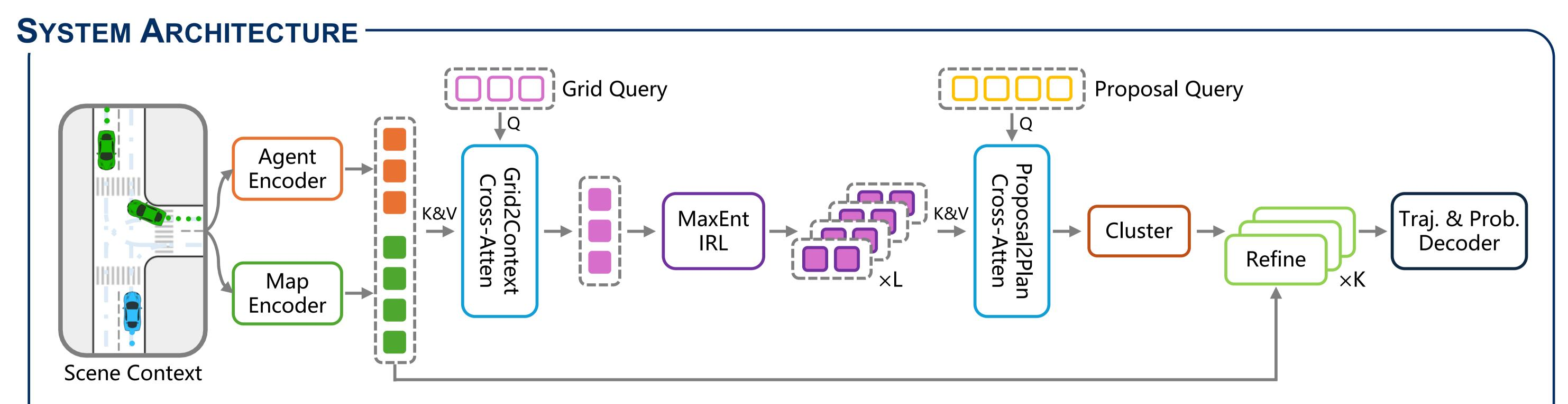
The scene context features are first extracted using agent & map encoders and then aggregated to the grid-shaped queries.
