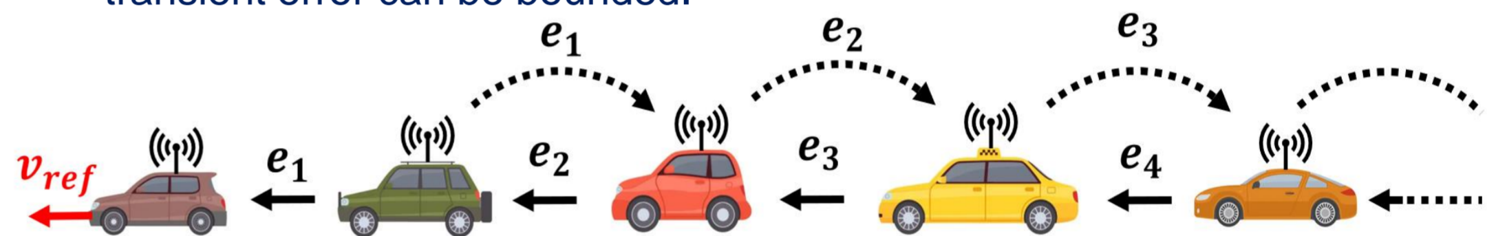
Figure 2: Communication structure of serial protocol
